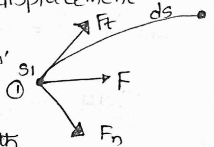
Let  $v_1$  &  $v_2$  be the velocities of the particle at position ① & position ②. and the corresponding displacement  $s_1$  &  $s_2$  respectively.
