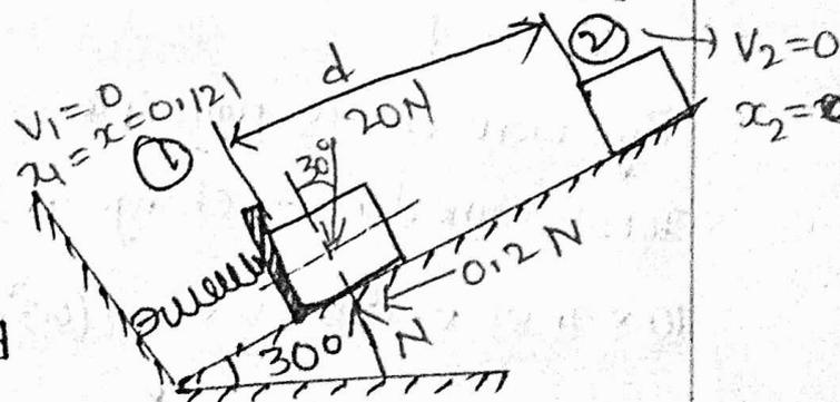
A block 'p' of weight 50 N is pulled so that the extension in the spring is 10 cm. The stiffness of the spring is 4 N/cm & the Co-efficient of friction b/w the block & the plane is  $\mu = 0.3$ . find
