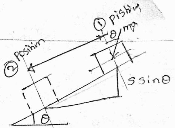
Work done = component of weight in the direction of displacement  $\times$  Displacement.
