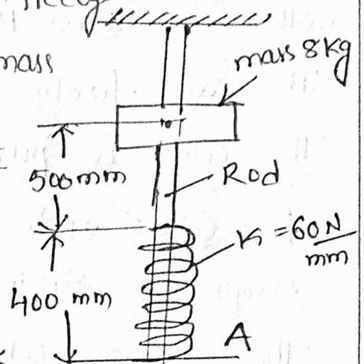
Determine the velocity of block when spring compressed through 20 mm. The free length of the spring is 400 mm.
